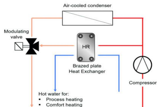
The solution proposed by Euroklimat for Total Heat Recovery is a modulating solution, based on the concept that the recovery load may vary during the function of the unit and, as a consequence, there could be:
