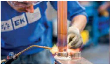
The next stop is at refrigerant circuit assembly station. Here the pipes of the circuit are assembled and brazed welded, which will connect the various elements of the unit, such as compressor(s), condenser(s), evaporator(s), etc. The refrigerant circuit is specifically designed in order to minimize load losses and to avoid capacity reduction. The circuit is entirely made of copper tube brazed with silver alloy and it is isolated on the suction part, in order to avoid condensation.
