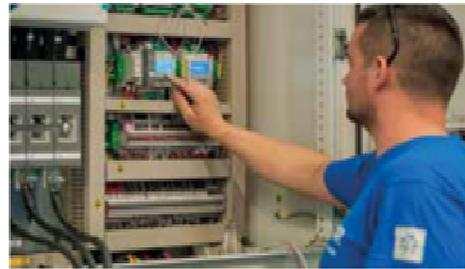
Once completed the refrigeration and water circuit, we perform the electrical wiring and the connection between electric board and compressor, fan, pump, etc. Each unit is equipped with electric panel, built, wired and fully tested at the factory. Wiring numeration and optimized layout facilitate troubleshooting. The installed components are identified by nameplates to better identify the application and the type of action.
