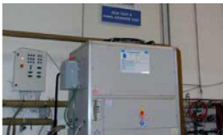
The production cycle draws to a close at the running test station. Here all models are individually tested in order to check correct operation, refrigerant charge and settings of microprocessor.
