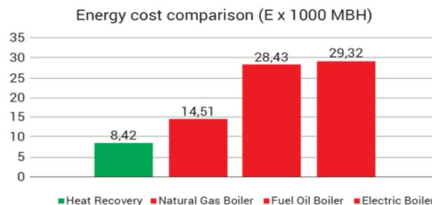
**Reduced Environmental Emissions**: energy recovery not only reduce operating costs, but also reduce emissions to the environment. Heat recovery systems allows the reduction of heat generated by burning fossil fuels (such as natural gas), and consequently the reduction of site emissions.
