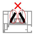
Buffer foam must be completely Fit into track slot Must not be exposed and clamped
