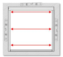
The above dimensions shall prevail, and the error between the middle and lower dimensions and the upper dimension shall not be greater than 3mm
