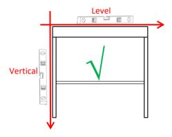
The distance between the upper and lower ends of the tracks is equal Error ≤ 3mm
