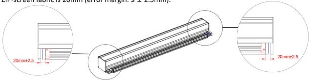
(2) If one side does not meet the size standard (20 mm), pull out the ZIP screen completely and then adjust the fabric sideways so that it is centered.
