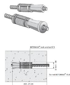
(Minimum value for B 25 concrete; deeper when anchoring in rock)
