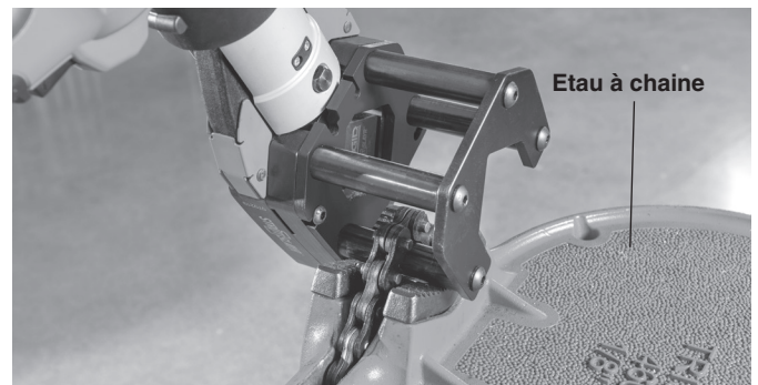
Figure 5 – Strut Shear Head Mounted in Chain Vise
