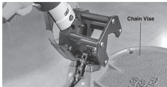
Figure 5 – Strut Shear Head Mounted in Chain Vise
