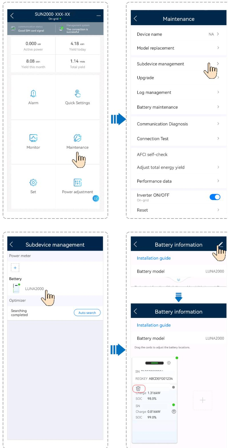
When the EMMA is used for networking, **connect the EMMA on the app**, tap **Monitor** on the home screen, select the connected inverter, choose **Maintenance > Subdevice management**, tap the ESS icon, and delete the offline Energy Storage Module.
