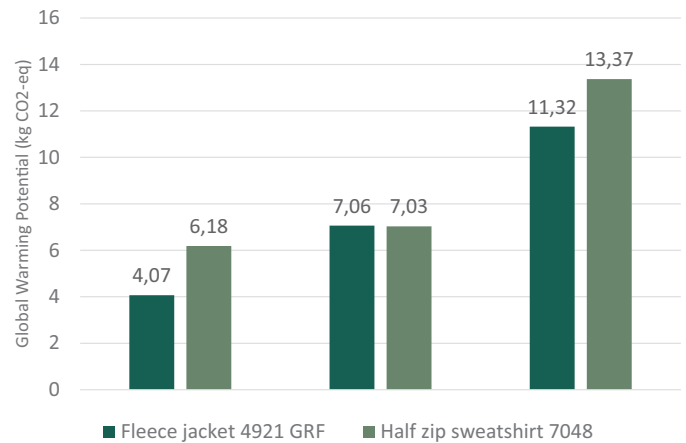
Figure 3. The Global Warming Potential of Fleece jacket 4921 GRF and Half zip sweatshirt 7048 SHV. Figures for one sweater of 500 grams respective 400 grams.
