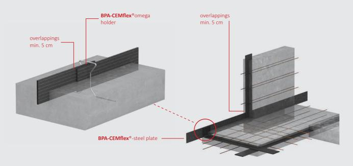
BPA-CEMflex® VB Plate Waterstop can be installed in two simple methods: either by fixing it to the steel reinforcement pre-pour using BPA-CEMflex® Omega Holders or alternatively by pushing the plate into the first pour of concrete to a depth of at least 30 mm, allowing the remainder of the plate to be covered by the next pour of concrete. To connect elements simply overlap the plates by 5 cm and
