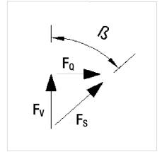
Loading capacity is the maximum load according to the "Safety rules for lifting sockets and systems for precast concrete elements". The figures include all safety factors for rope failure (4), steel failure (3) and concrete failure (3).
